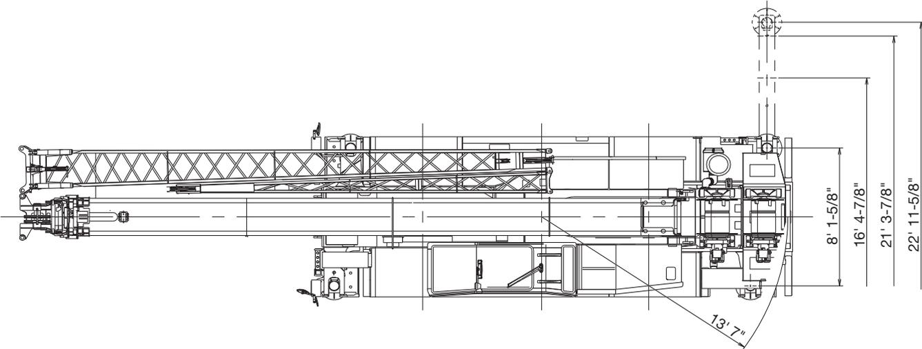
Dimension is with boom angle at -0.8 degree.
