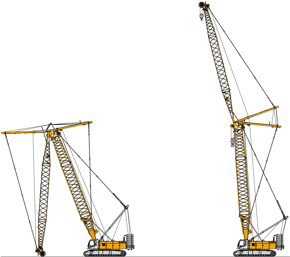
Erecting of main boom and luffing jib
